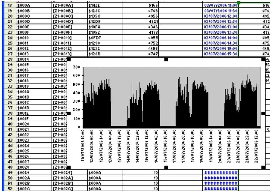
**Exemple 1:** Storage of active power (kWh) integrated on 10 minutes and 62 days. With internal synchronisation (internal clock) and reading by communication.
