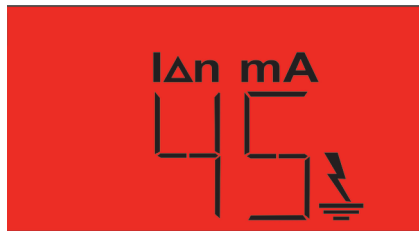
Figure 11: Trip current screen (Example: 45mA trip current)
