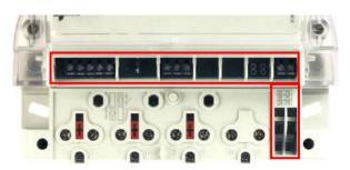
Fig. 33: Position of inputs and outputs on MT372 meter front view
