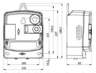
Fig. 5b: Overall and fixing dimensions of a meter fitted with a short terminal cover
