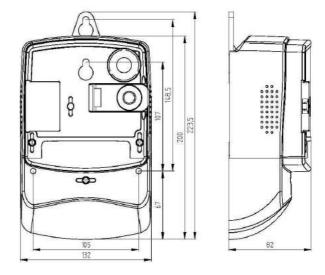
Fig. 5c: Overall and fixing dimensions of a meter with BS terminal block fitted with a long terminal cover
