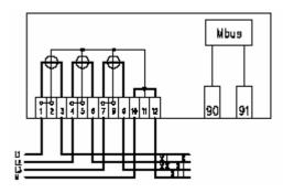
Fig. 47: Connection diagram of MT371 meter with M-Bus communication interface
