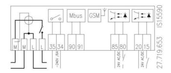
Fig. 46: Connection diagram of ME372 meter with GSM/GPRS modem and BS terminal block
