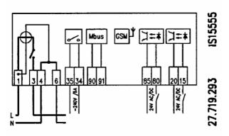
Fig. 45: Connection diagram of ME372 meter with GSM/GPRS modem
