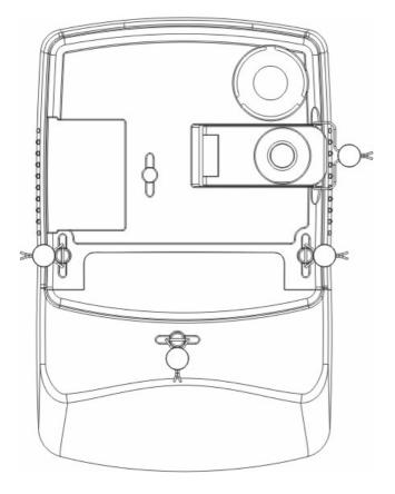
Fig. 37: ME37y meter position of the seals
