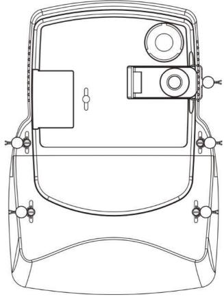
Fig. 38: MT372 meter position of the seals
