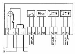
Fig. 43: Connection diagram of ME371 meter
