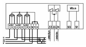
Fig. 48: Connection diagram of MT371 meter with outputs and M-Bus communication interface
