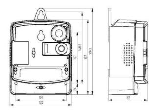
Fig. 5d: Overall and fixing dimensions of a meter with BS terminal block fitted with a short terminal cover
