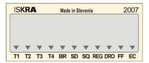
Fig. 31: Display legend, Mx372 (GSM/GPRS, RS485)
