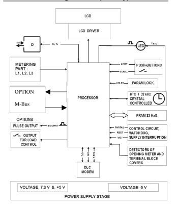
Fig. 19: MT371 meter block diagram
