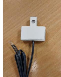
The LPS is provided with a sticky pad which is used to attach it to the meter.
