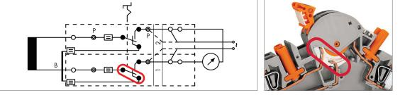
The measuring instrument is electrically disconnected from the transformer. In this position, if necessary, external voltage can be applied via sockets, or the 2nd CAGE CLAMP® connection for relay testing in transformer protection circuits.
