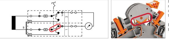
In position "I", the measuring instrument is connected to the transformer.
